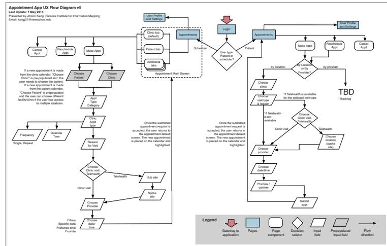
FIGURE 5: A sample UX flowchart that served as the blueprint for communicating the site/module structure and content organization.
